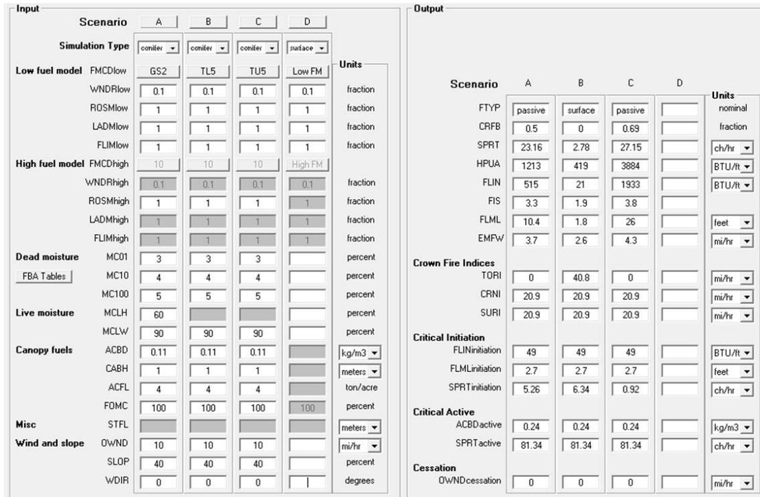
**Figure 27.** NEXUS fire modeling system. NEXUS facilitates in depth fire behavior critique and is particularly useful in assessing the environment conditions required to transition surface fire to crown fire based on fire behavior fuel model and canopy base height values.
