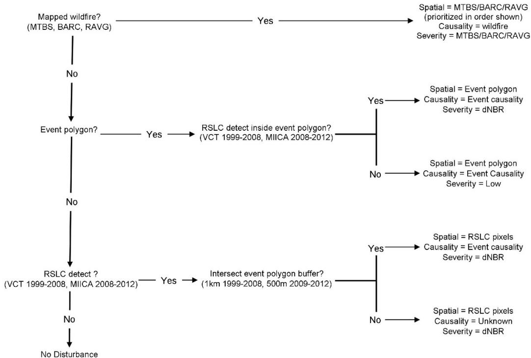
**Figure 5.** The LANDFIRE disturbance mapping process. LANDFIRE disturbance data are developed through a multistep process that incorporates Landsat satellite imagery, local agency derived disturbance polygons, and other ancillary data.
