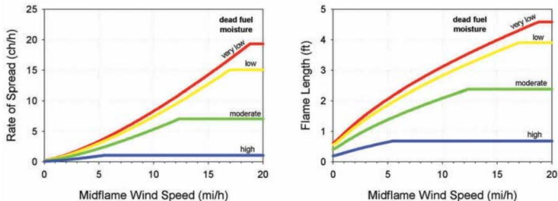
**Figure 13.** Differences in rate of spread and flame length by dead fuel moisture content and wind speed for fuel model Timber-Understory 1 (Low Load Dry Climate Timber-Grass-Shrub; Scott and Burgan 2005).
