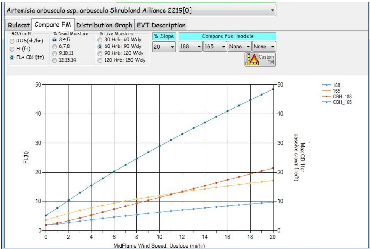
**Figure 16.** LANDFIRE Total Fuel Change Tool compare fuel model tab. This allows the user to calculate the critical canopy base height needed for crown fire initiation for different combinations of fire behavior fuel model, fuel moisture, and wind speed.
